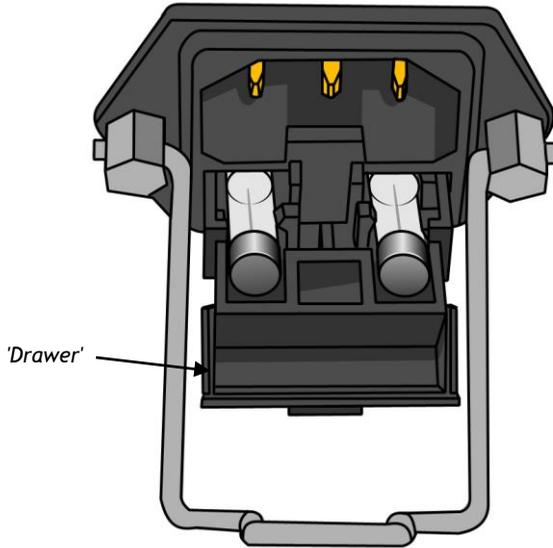
Unplug and remove IEC cable. Using a flat-bladed screwdriver, or similar, pull forward the 'drawer' containing the fuses. Hinge down the front of the holder. Lift the fuses by pushing them through the holes below.
