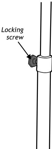
The telescopic extension is released for raising and lowering, and locked by the locking screw at the rear of the up-stand.
